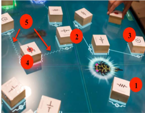
Figure 1. Players assemble virtual circuits using wooden blocks that represent resistors (1), batteries (2), timers (3), and different colored LEDs (4). Participants make connections (depicted as lines on the tabletop - 5) by bringing the positive and negative terminals of the blocks (displayed by the table) in contact with one another. Creating a successful circuit causes the LEDs to glow and lures fish attracted to that light.
