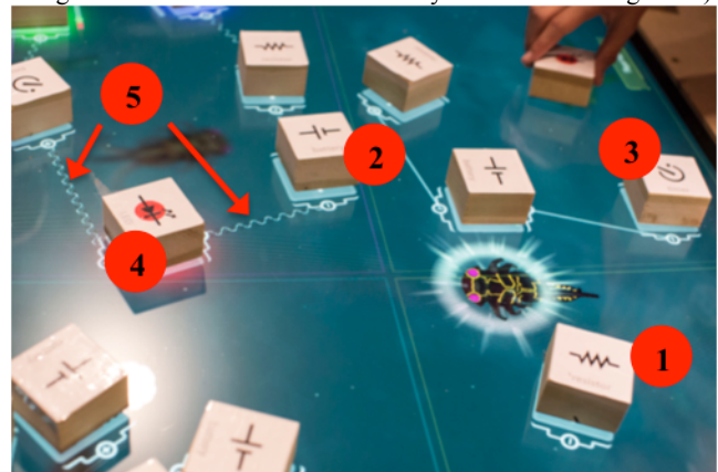
Figure 1. Visitors assemble virtual circuits using wooden blocks that represent resistors (1), batteries (2), timers (3), and different colored LEDs (4). Visitors make circuit connections (depicted as lines on the tabletop - 5) by bringing the positive and negative terminals of the blocks (augmentations displayed by the table) in contact with one another. Creating a successful circuit (one that has the correct ratio of resistors, batteries, and LEDs) causes LEDs to glow and lures creatures attracted to it for cataloging.
